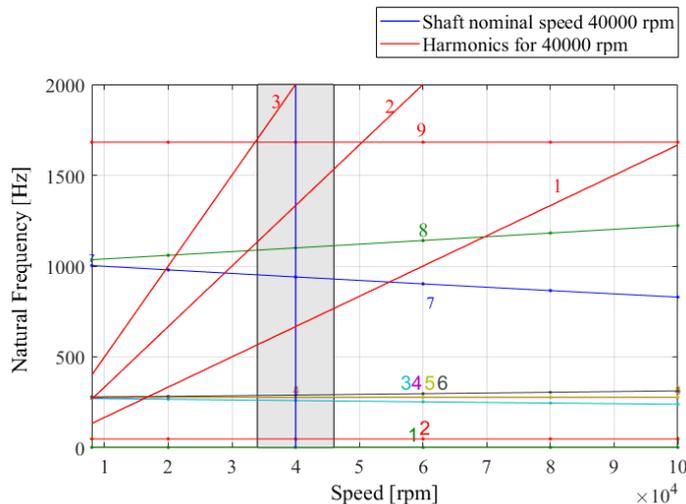
**Figure 5** Campbell diagram of the rotor of a 30 kW microturbine
